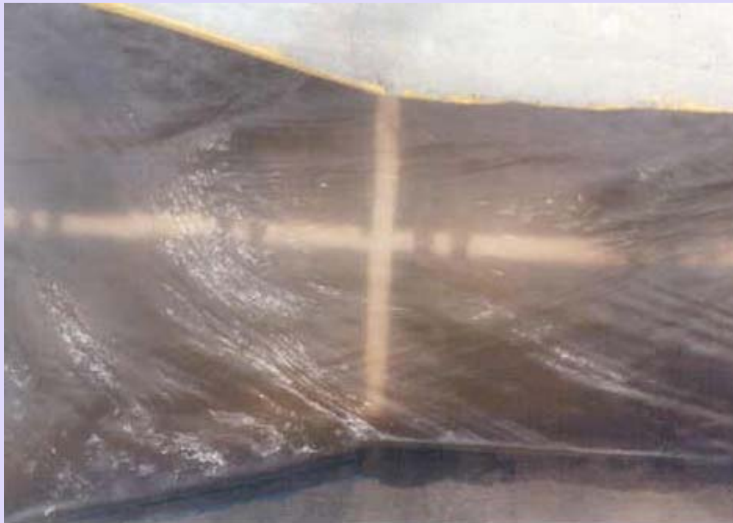
Super critical approach flow - Shocks can be seen
