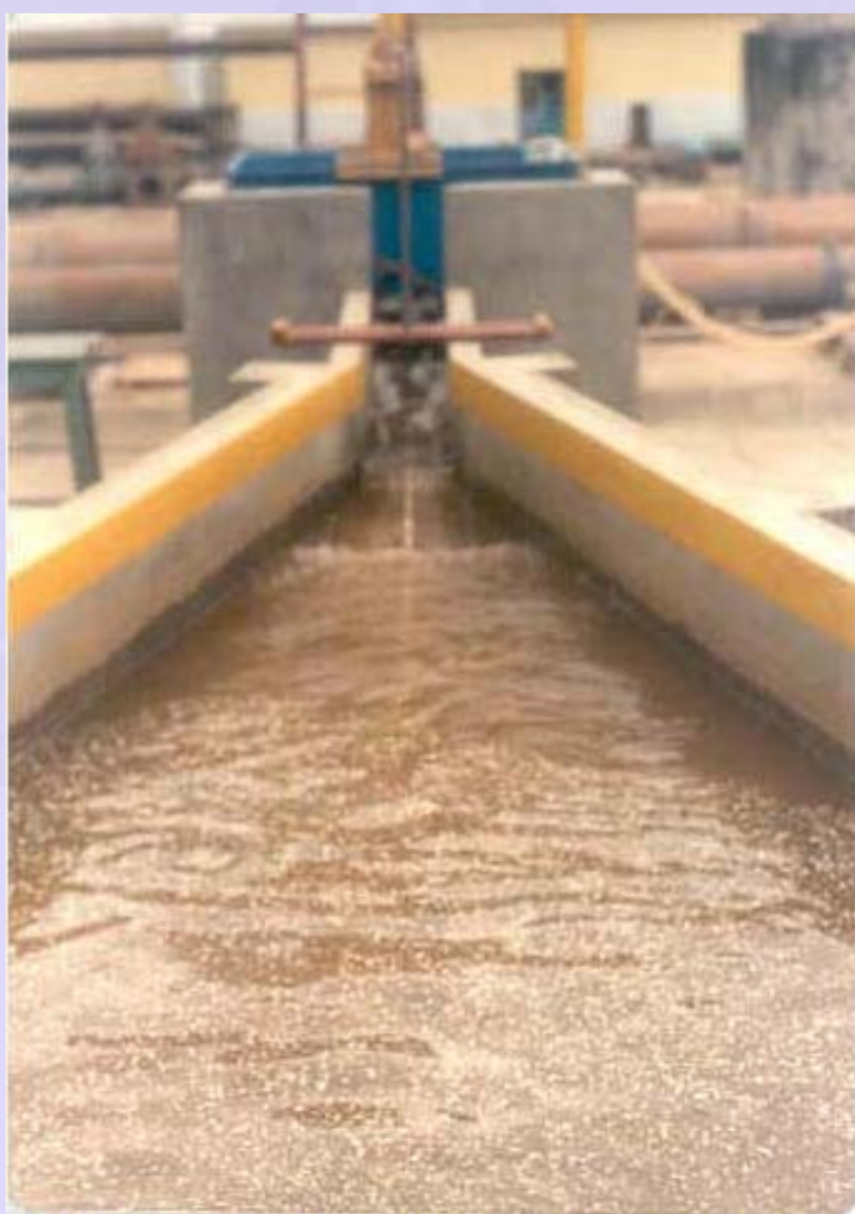
Jump in gradual expansion - looking upstream
